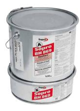
Two-component, epoxy-based construction resin used as primer and adhesion promoter for substrate preparation and for production of epoxy resin mortars. For production of synthetic resin mortars allowing early installation of coverings, used in conjunction with Sopro EEK 871 epoxy screed aggregate (achieving grade SR-C25-F7 to DIN EN 13 813) or with Sopro DEK 872 pervious screed aggregate (achieving grade SR-C20-F6 to DIN EN 13 813).
