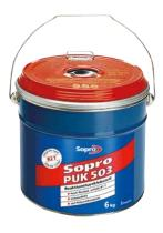
Light-coloured, waterproof, rapid-set, solvent-free, two-component reaction resin adhesive, meeting R2 T requirements to DIN EN 12004, for installation of ceramics and natural stone units.
